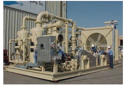
2004 West Africa installation. Dual rotary vane – 4 MMSCFD @ 40 psi
