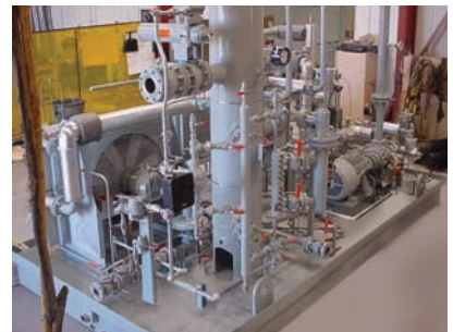
2004 Gulf of Mexico installation. Rotary screw 300 MCFD @ 250 psig
