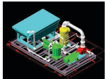
2004 Gulf of Mexico installation. Rotary screw 300 MCFD @ 250 psig
